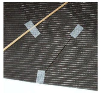
edge. Draw a straight line beginning at the trailing edge and extending 5" (127mm) toward the nose. Repeat for the other side of the kite. These lines are the locations for the kite's battens.
