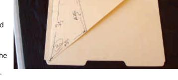
• The triangle shape you've drawn is the full sized shape of 1/2 of the kite skin. Cut out the triangle using a straight edge and razor knife. The triangle is your kite skin template.
